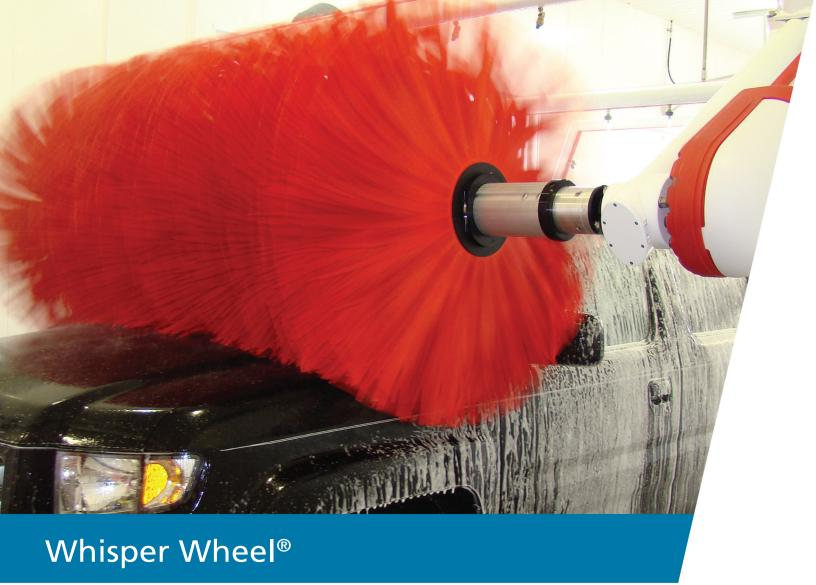
Designed as a dedicated horizontal surface washer, the Whisper Wheel® excels at cleaning hoods, roofs and trunk lids — all while providing a super-quiet customer experience. The uniquely shaped Neotex<sup>™</sup> closed-cell foam wash 'fingers' provide superior wash penetration with vastly reduced in-car noise levels.
