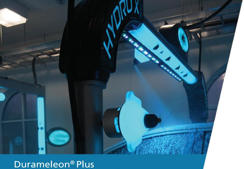
The illuminated Durameleon® Plus Arch Series is built to perform — with the available patented Twist-N-Flip $^{\text{TM}}$  action of the top and side nozzles. Delivering the most complete application coverage ever from one arch, this feature uses a single air cylinder to synchronize all 3 manifolds, for complete coverage of the vehicle front, sides, top, mirrors, and back — every time.
