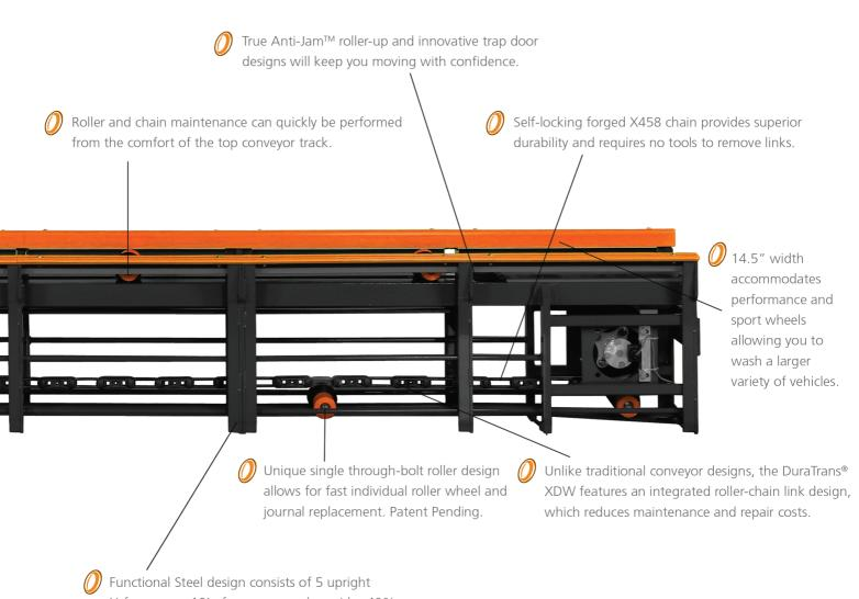
Functional Steel design consists of 5 upright H-frames per 10' of conveyor and provides 40% more structural integrity than competitive designs.
